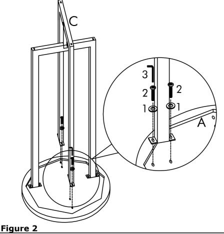
Connect Lower Leg Frame (C) to assembled unit on Figure 1 with Bolts (2) and Flat Washers (1).
