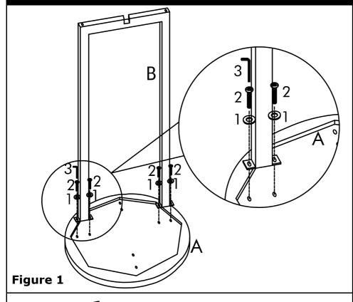
Connect Upper Leg Frame (B) to Top Frame (A) with Bolts (2) and Flat Washers (1).
